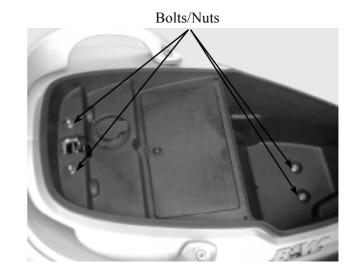
Remove the hand rail right and left lock hex bolts.
