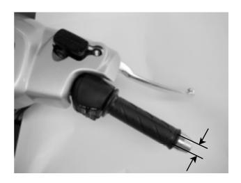
Major adjustment of the throttle grip free play is made with the adjusting nut at the carburetor side. Adjust by loosening the lock nut and turning the adjusting nut.
