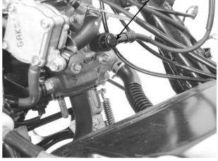
Remove the spark plug cap. Remove the two joint lock nuts on the front of the exhaust muffler and then remove the two exhaust muffler lock bolts.
