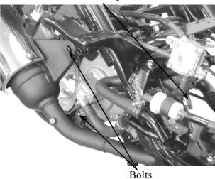
Remove the spark plug. Remove the cylinder head bolts and the
