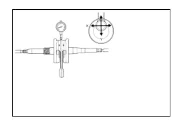
Measure the crankshaft runout.
