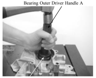
Bearing Outer Driver, 37x40mm Bearing Driver Pilot, 17mm
