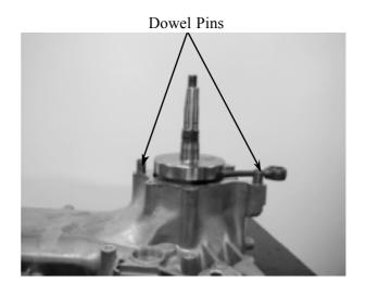
Assemble the crankcase halves.
