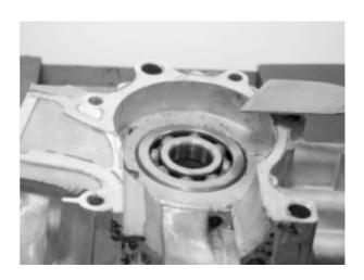
Drive a new crankshaft bearing into the right crankcase.
