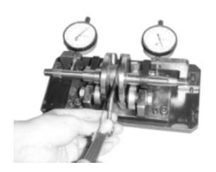
Measure the connecting rod big end radial clearance at two points in the X and Y directions.
