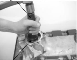
Bearing Outer Driver, 42x47mm Pilot, 20mm
