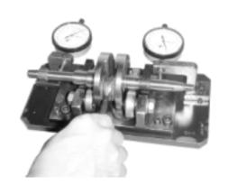
Check the crankshaft bearings for excessive play.
