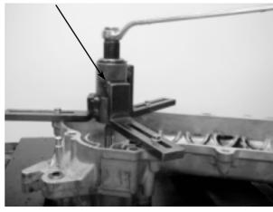
Remove the remaining bearing on the crankshaft side using the universal bearing puller.
