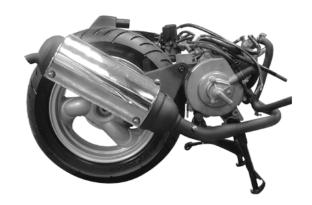
Remove the three bolts and the water pump cover, gasket and two dowel pins.
