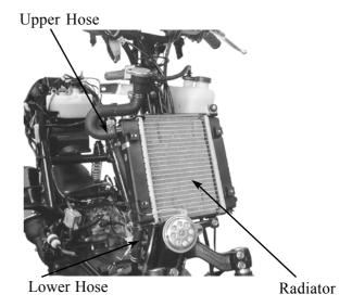
Remove the two bolts and two nuts on the radiator.
