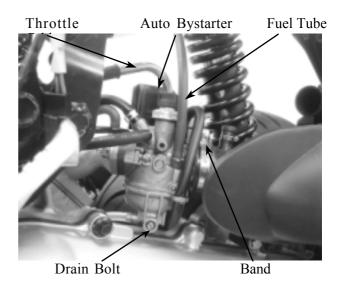
Remove the two carburetor lock nuts. Remove the carburetor and water hose.
