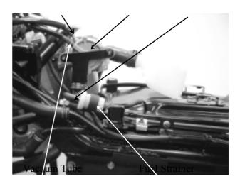
Measure the fuel pump output. Start the engine and disconnect the fuel outlet tube and place a clean container under the tube to check the fuel output.
