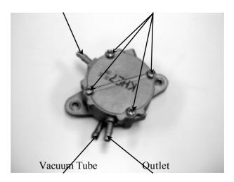
Disassemble the fuel pump.
