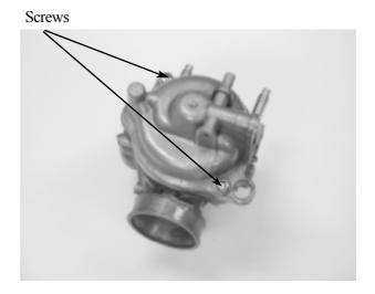
Remove the screw and O-ring. Remove the float pin, float and float valve.
