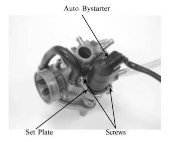
Check the auto bystarter valve and needle for wear or damage. Check the O-ring for wear or damage.
