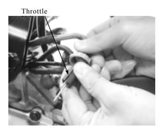
Remove the throttle valve spring, carburetor cap and rubber seal.
