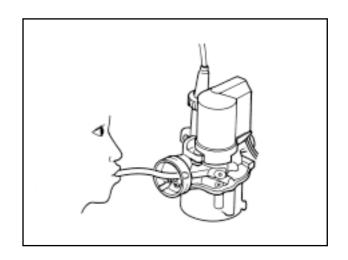
Connect the auto bystarter yellow wire to the battery positive (+) terminal and green/ black wire to the battery negative (-) terminal and wait 5 minutes. Connect a hose to the fuel enriching circuit and blow the hose with mouth. If air can be blown into the hose, the auto bystarter is faulty and replace it with a new one
